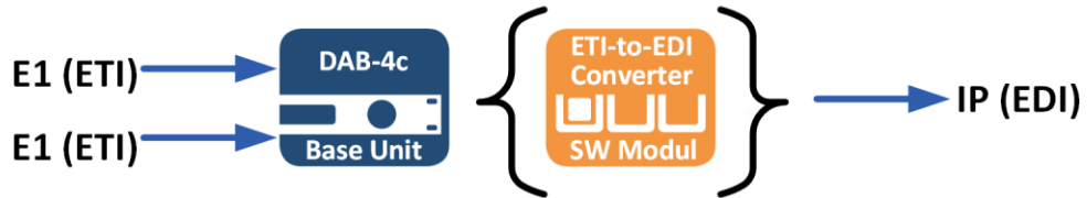
ETI-to-EDI converter with ETI Redundancy
