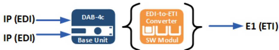
EDI-to-ETI converter with EDI PFT Seamless Switching
